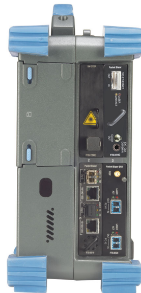
The FTB-8510G Packet Blazer 10 Gigabit Ethernet Test Module is housed in the FTB-400 Universal Test System, EXFO's rugged, all-in-one portable platform. Also shown in the platform, the FTB-8510 Packet Blazer Ethernet Test Module and the FTB-8120/8130 Transport Blazer Next-Gen SONET/SDH Test Module.
